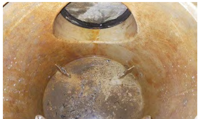
MetaLine-protected strainer after five years of operation
