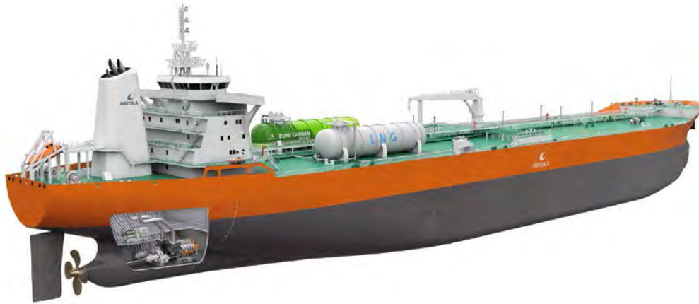
The new design is based on a single engine for both propulsion and electric power generation
