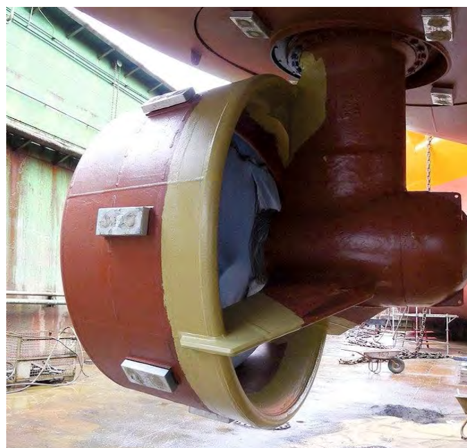
The high-revving propeller carries a huge flow of water, which leaves cavitation and erosion marks, especially on the suction-side edge and on the supports of the nozzle
