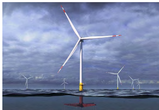
An artist's rendering of the 12-MW floating wind turbine concept GE Research and Glosten are jointly designing
