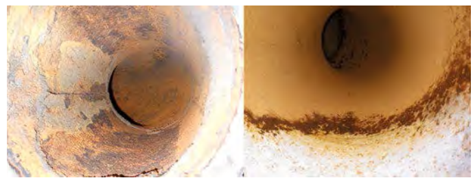
Seawater pipe before repair and coating and five years later. Only rust particles from unprotected areas have settled.
